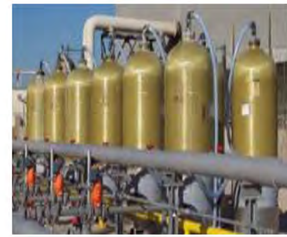
Fluidized Bed Reactor
