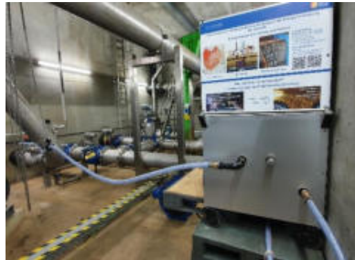
Deployment at a water treatment plant for radioactive mine water (T = 26 °C !)
