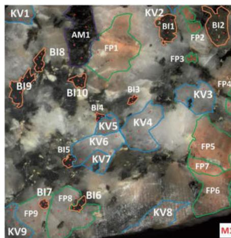
Minerals in Mórág granite rock, identified with 92% accuracy by RF method
