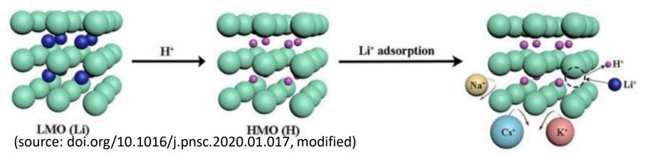
Lithium ions are introduced into the manganese compound to form a spinel structure through heat treatment. Subsequently, the lithium ion is extracted from the spinel structure by acid treatment, with a proton replacing Li<sup>+</sup> to form a lithium ion sieve without changing the crystal structure. In the presence of multiple ions, the lithium ion sieve has the ability to screen and remember a target ion, which is called the 'ion sieve effect'.
